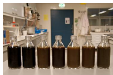
Photo 2. Mineral concentrates from different reverse osmosis installations.
