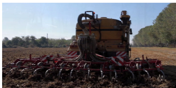
Figure 2. Digestate injection application on agricultural land.
