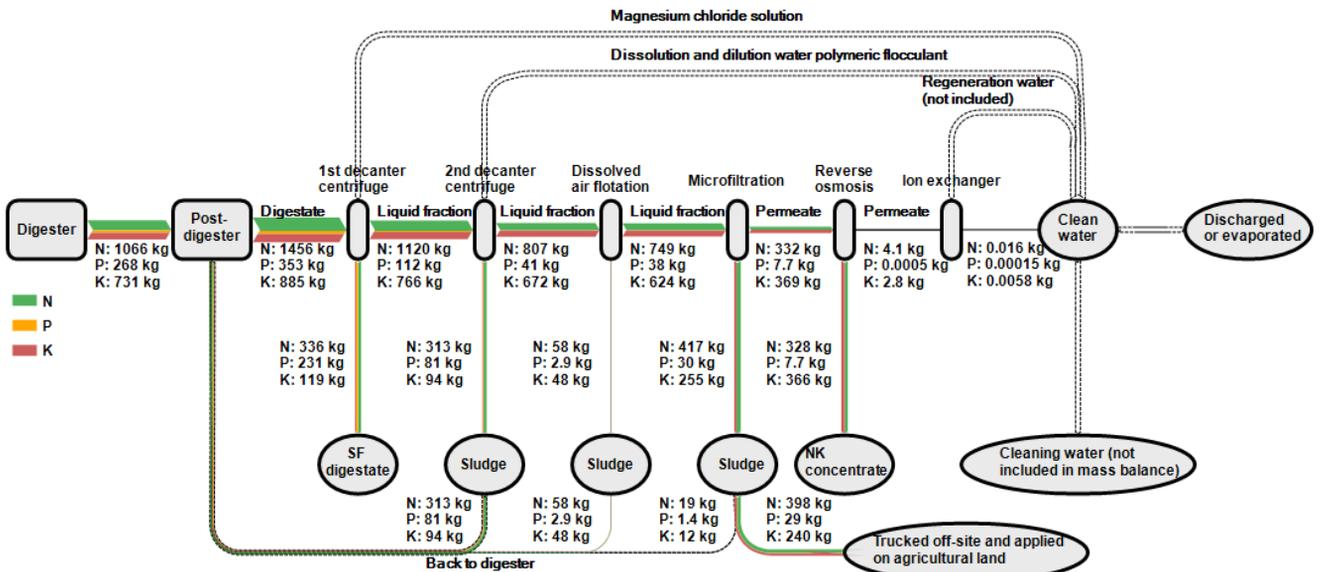
Figure 4 Total nitrogen (N), phosphorus (P) and total potassium (K) mass flows at Groot Zevent Vergisting for the period October 2019–January 2019. Values are expressed in kilograms per day (kg d<sup>-1</sup>).
