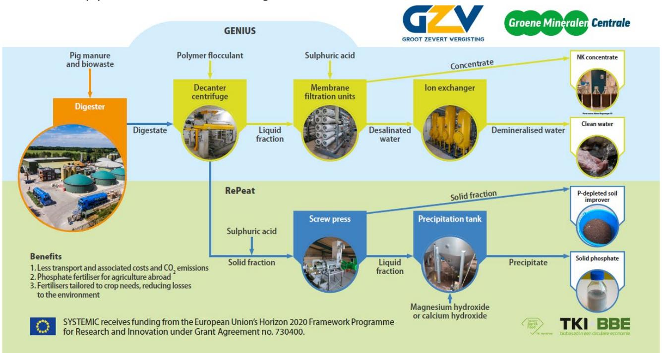
Figure 2. Simplified process scheme of the biogas plant of Groot Zevert Vergisting.
