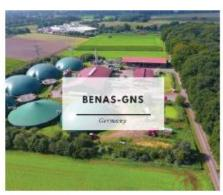
The Benas-GNS demonstration plant is located in northern Germany, near Bremen. The plant treats over 80kt of com sitage, chicken manure and food waste per year and has the capacity to process up to 170kt per year. Currently the plant produces biogas, mineral N, calcium carbonate and organic fertilisers. The remaining digestate is spread on the company's 35,000ha of farmland.
