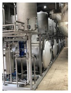
Photo of the Evaporator-condensator installation at AmPower (Pittem, Belgium).
