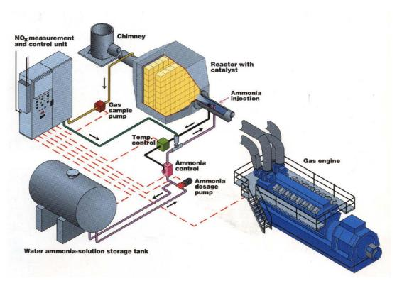
Figure I-3.SCR in gas engine. Source: Wärtsila Nederland
