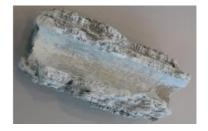
Figure II-3. Struvite depositions in the pipes of the sludge holding tank.
