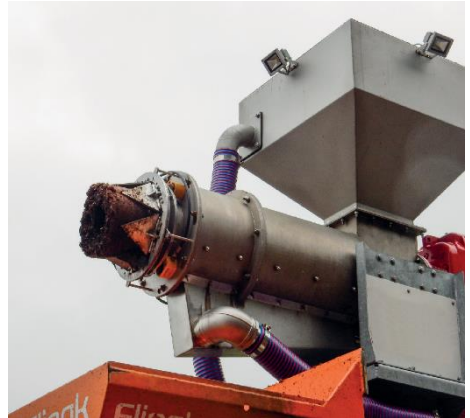
Figure 2-5 Screw press. Source: (Gorissen and Snauwaert 2018)
