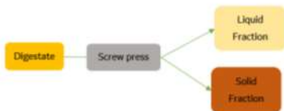
Figure 2-4 Scheme of separation of digestate with screw press and recovery rates.
