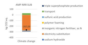
The bar goes from -300 to +100, the numeric value is -267.09 kg  $CO_2$ -eq showing savings of 267.09 kg  $CO_2$ -eq per ton of substrate treated compared to the reference scenario. The negative impact is transport, the main positive impacts are renewable electricity and substitution of mineral N and P fertilisers.
