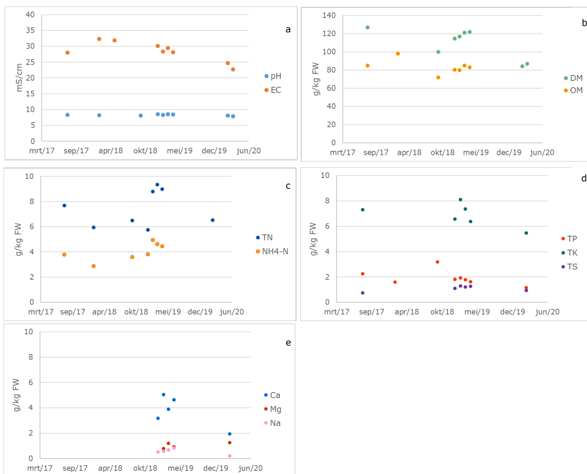
Figure 6-7 Composition (in fresh weight) over time of digestate produced at BENAS for the period August 2017 – February 2020: a) pH and EC; b) dry matter (DM) and organic matter (OM); c) total nitrogen (TN) and ammoniacal nitrogen ( \text{NH}_4\text{-N} ); d) total phosphorus (TP), total potassium (TK) and total sulphur (TS); e) calcium (Ca), magnesium (Mg) and sodium (Na).
