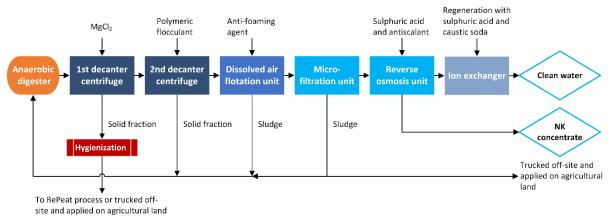
Figure 1.4 Process flow diagram of the GENIUS installation at the demonstration plant Groot Zevert Vergisting, including locations of chemical addition and the major return flows (as configured in May 2020).
