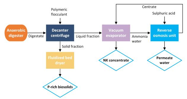
*Figure 2.1 Process flow diagram of the initially envisaged NRR facility of the demonstration plant AM-Power.*
