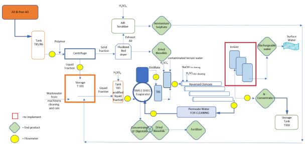
Figure 2.5 Process flow diagram of the final NNR facility of the demonstration plant AM-Power.
