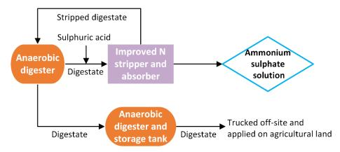
Figure 3.1 Process flow diagram of the final NNR facility of the demonstration plant Acqua&Sole.
