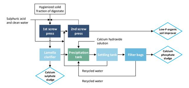
Figure 1.3 Process flow diagram of the RePeat installation at the demonstration plant Groot Zevert Vergisting including locations of chemical addition and the major return flows (as configured in May 2020).
