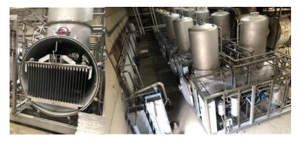
*Figure 2.2 The vacuum evaporator installed at the demonstration plant AM-Power (2019).*
