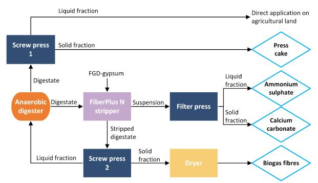
Figure 4.1 Process flow diagram of the final NNR facility of the demonstration plant Benas.
