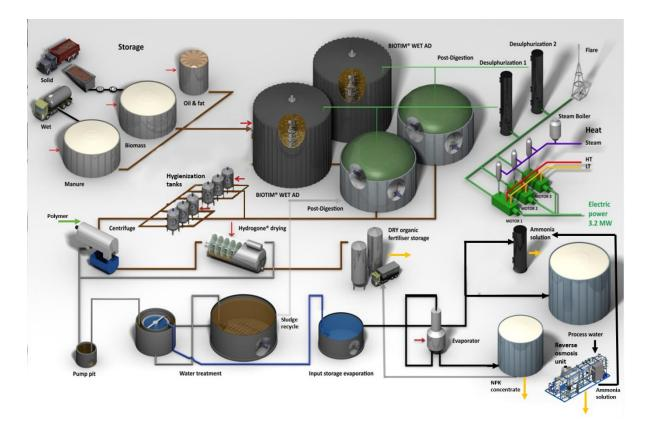
Figure 6.1. Process flow diagram of the final NNR facility of the demonstration plant Waterleau New Energy. Yellow arrows indicate final products, red arrows indicate locations where heat is reused (steam or hot water), HT: high temperature water (95 °C), LT: low temperature water (40 °C).
