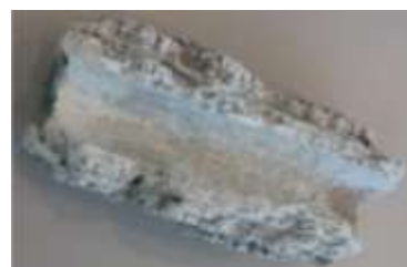
Figure III-3. Struvite depositions in the pipes of the sludge holding tank.
